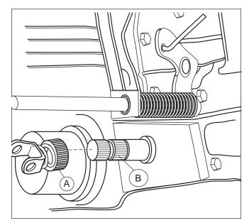
Figure 2 A. Drive Shaft Locking Collar B. Transmission Shaft
